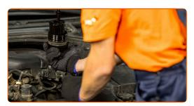
19 Remove the filter element from the filter housing.
