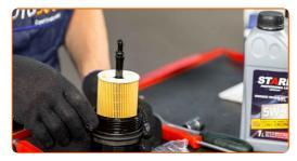
Screw the new filter into its place. Use the 86/16 F socket. Use a torque wrench. Tighten it to 23 Nm torque.
