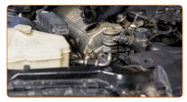
Unscrew the oil filter. Use the 86/16 F socket. Use a ratchet wrench.
