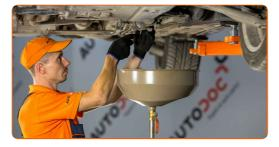
Loosen the fuel filter mounting. Use a drive socket #10. Use a ratchet wrench.
