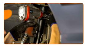
Tighten the fastener connecting the stabilizer link to the shock strut. Use a drive socket #17. Use a torque wrench. Tighten it to 60 Nm torque.
