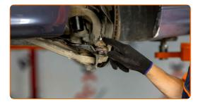
Unscrew the end fastening nut to the steering knuckle. Use a drive socket #19. Use a ratchet wrench.
