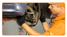
Tighten the fastening nut connecting the tie rod end to the steering knuckle. Use a drive socket #18. Use a torque wrench. Tighten it to 65 nm torque.
