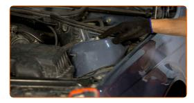
Unscrew the top fastening of the shock strut mount. Use a drive socket #13. Use a ratchet wrench.
