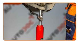
Screw the fastener connecting the ball joint to the steering knuckle. Use a combination spanner #19. Use a torque wrench. Tighten it to 65 Nm torque.
