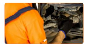
Tighten the fastener connecting the stabilizer link to the shock strut. Use a combination spanner #16. Use a drive socket #17. Use a torque wrench. Tighten it to 60 Nm torque.
