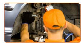
Unscrew the fastener connecting the stabilizer link to the stabilizer bar. Use a combination spanner #16. Use a drive socket #17. Use a ratchet wrench.
