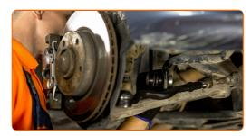
Tighten the fastener connecting the stabilizer link to the stabilizer bar. Use a combination spanner #16. Use a drive socket #17. Use a torque wrench. Tighten it to 60 Nm torque.
