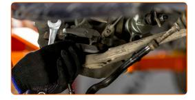
Treat the retaining bracket that secures the brake hose and the wiring harness. Use WD-40 spray.
