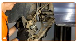
Connect the lower arm to the steering knuckle.
