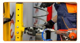
Remove the shock absorber dust cap and the bump stop.
