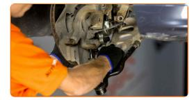
Unscrew the brake hose fastening bracket from the shock strut. Use a drive socket #18. Use a ratchet wrench.
