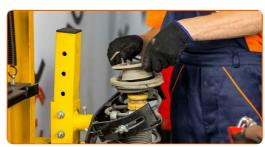
Tighten the shock strut piston rod nut. Use a drive socket #22. Use HEX No.H6. Use a torque wrench. Tighten it to 64 Nm torque.
