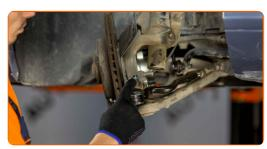
Unscrew the end fastening nut to the steering knuckle. Use a drive socket #19. Use a ratchet wrench.
