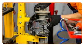
Remove the shock strut mount cap. Use a flat screwdriver.
