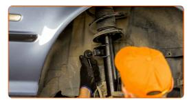
Tighten the fastener connecting the stabilizer link to the shock strut. Use a drive socket #17. Use a torque wrench. Tighten it to 60 Nm torque.
