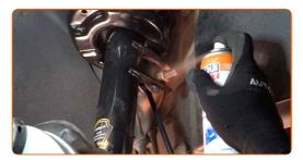
Treat the surface where the brake disc contacts the wheel rim. Use copper grease.
