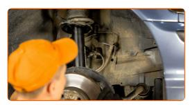
Tighten the brake hose fastening bracket to the shock strut. Use a drive socket #18. Use a ratchet wrench.
