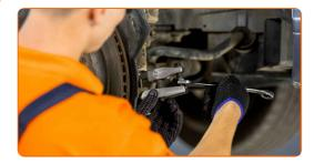
Clean the fastener that connects the ball joint to the steering knuckle. Use a wire brush. Use WD-40 spray.
