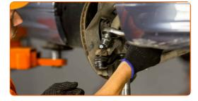
Fasten the brake hose on the strut.
