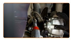
Disconnect the ABS sensor wiring.
