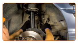
Remove the support from under the arm.
