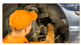
Disconnect the ball joint from the steering knuckle. Use a ball joint puller. Use a crowbar.
