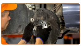
Tighten the fastener of the wheel hub bearing. Use a drive socket #46. Use a torque wrench. Tighten it to 290 nm torque.
