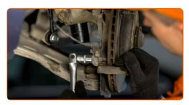
Remove the caliper bracket.
