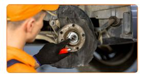
Unscrew the hub bearing mounting. Use a drive socket #46. Use a tap wrench.
