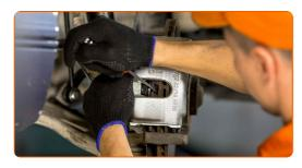
11 Remove the brake caliper.
