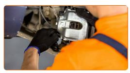
Undo the brake bleeder screw. Use a combination spanner #9.
