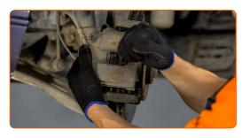
14 Remove the brake caliper.
