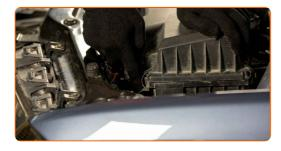
Lock the retaining clips of the air filter housing cover.
