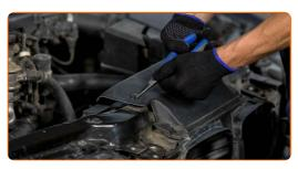
Detach the air duct housing from the air filter housing.
