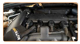
Detach the connector from the ignition coil.
