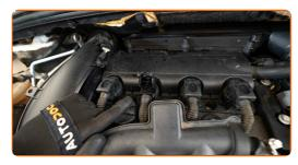
Detach the connector from the ignition coil.
