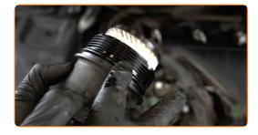
Install a new oil filter housing cover and tighten it. Use a drive socket #27. Use a torque wrench. Tighten it to 25 Nm torque.
