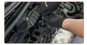
Screw new spark plugs and tighten them. Use the spark plug socket #14. Use a torque wrench. Tighten it to 25 nm torque.
