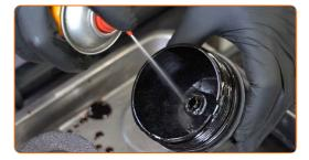
Install a new O-ring to its mounting seat on the filter cover.
