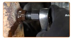
Treat the oxygen sensor. Use copper grease.
