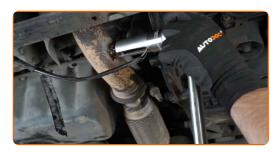
6 Remove the oxygen sensor.
