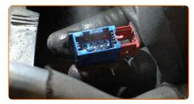
13 Attach the oxygen sensor connector.
