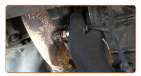
Tighten the oxygen sensor fastener. Use a combination spanner #22. Use a torque wrench. Tighten it to 47 Nm torque.
