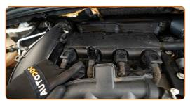
Detach the connector from the ignition coil.
