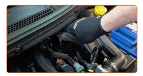
Tighten the clamp fastening the engine air filter housing to the throttle body. Use a drive socket #7.
