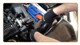
Remove the air filter housing.
