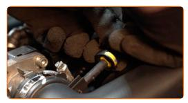
Unscrew the clamp fastening the engine air filter housing to the throttle body. Use a drive socket #7.
