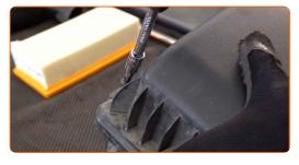
Reinstall the air filter housing.
