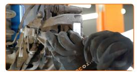
12 Remove the brake caliper.
