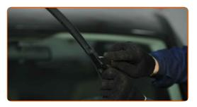
Remove the blade from the wiper arm.
