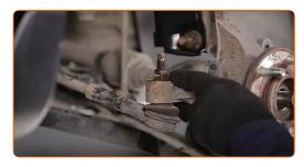
Unscrew the end fastening nut to the steering knuckle. Use a combination spanner #18. Use a ratchet wrench.
