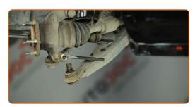
Detach the driveshaft from the steering knuckle. Use a pin punch. Use a hammer.
