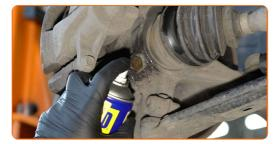
Unscrew the brake caliper bracket fasteners. Use a drive socket #18. Use a tap wrench. Use a ratchet wrench.
