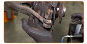
Tighten the fastening nut connecting the tie rod end to the steering knuckle. Use a combination spanner #18. Use a torque wrench. Tighten it to 75 nm torque.
