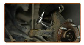
Remove the ABS sensor from the steering knuckle. Use a flat screwdriver.
