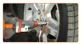
Lower the car and working in a cross order, tighten the wheel bolts. Use wheel impact socket #19. Use a torque wrench. Tighten it to 135 nm torque.
