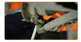
Remove the fastening bolt.
