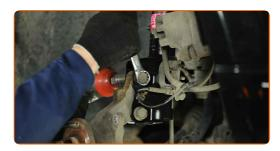
Remove the fastening bolts. Use a pin punch. Use a hammer.
