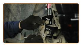
57.1 Install the ABS sensor on the steering knuckle and secure it.
