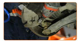
Treat the fastener connecting the tie rod end to the steering knuckle. Treat the steering knuckle fasteners. Treat the brake caliper bracket fasteners. Treat the fasteners connecting the control arm to the steering knuckle. Use copper grease.
