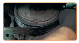
Rotate the crankshaft several times to check whether the new V-ribbed belt is working correctly. Use a drive socket #18. Use a ratchet wrench.
