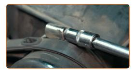
Detach the air duct clamp. Remove the air intake hose.
