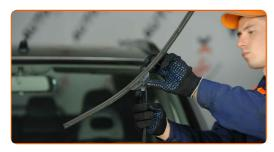
Remove the blade from the wiper arm.
