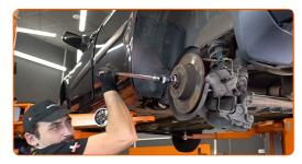
Remove the brake disc assemled with the wheel hub bearing.
