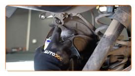
Unscrew the caliper bracket fastening. Use a drive socket #E16. Use a tap wrench.
