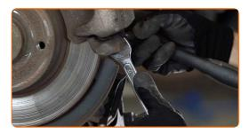
10 Remove the brake caliper.
