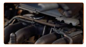
$\Lambda$  Remove the spark plug wire connectors from the spark plug wells. Use round-nose pliers.
