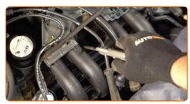
Unscrew the spark plugs. Use the spark plug socket #16.
