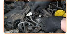
Unscrew the glow plugs. Use the spark plug socket #10. Use a ratchet wrench.
