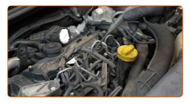
Detach the glow plug wiring connectors.
