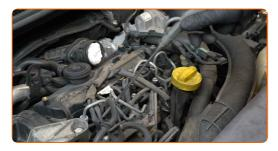
Detach the glow plug wiring connectors.
