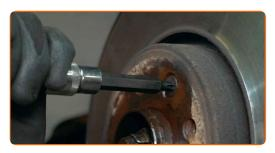
15 Remove the brake disc.
