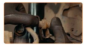
Treat all tie rod end connections. Treat the shock strut fasteners. Treat the fasteners of the ball joint. Use copper grease.
