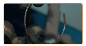
Press out the inner bearing race that is remaining on the hub. Use a bearing separator. Use a bush and bearing driver set.
