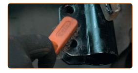
Clean the splines of the drive shaft CV joint. Use a wire brush. Use WD-40 spray.
