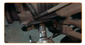
Disconnect the ball joint from the control arm. Use a crowbar.
