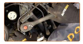
Take out the spark plugs. Use the spark plug socket #16.
