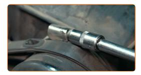
Detach the air duct clamp. Remove the air intake hose.
