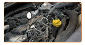
Detach the glow plug wiring connectors.
