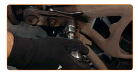
Screw in the fasteners connecting the suspension strut to the steering knuckle. Use a combination spanner #21. Use a drive socket #21. Use a ratchet wrench.
