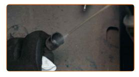
Attach the ABS sensor connector.
