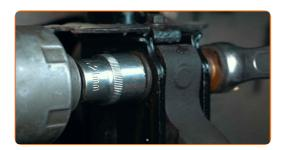
Tighten the lower fasteners connecting the shock strut to the steering knuckle. Use a combination spanner #21. Use a drive socket #21. Use a torque wrench. Tighten it to 170 Nm torque.
