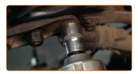
Tighten the fasteners connecting the ball joint to the control arm. Use a drive socket #18. Use a torque wrench. Tighten it to 75 nm torque.
