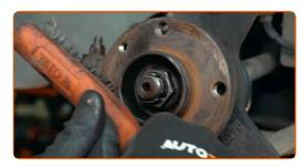
Treat the contacting surface. Use copper grease.
