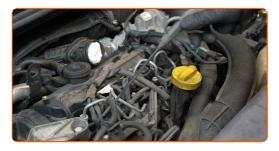
Detach the glow plug wiring connectors.
