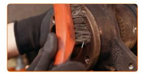
Treat the contacting surface. Use copper grease.
