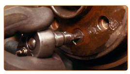
16 Remove the brake disc.
