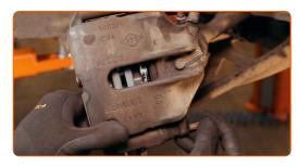
Tighten the brake caliper fasteners. Use a combination spanner #17. Use a drive socket #13. Use a torque wrench. Tighten it to 32 Nm torque.
