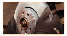
Tighten the brake disc fastening. Use Torx T40. Use a torque wrench. Tighten it to 14 Nm torque.
