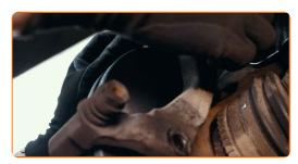
Tighten the brake caliper bracket. Use a drive socket #18. Use a torque wrench. Tighten it to 100 Nm torque.
