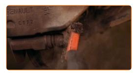
Unscrew the brake caliper fastening. Use a combination spanner #17. Use a drive socket #13. Use a ratchet wrench.
