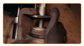
27 Install the brake caliper and fix it.
