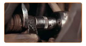
Remove the brake caliper.
