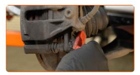
Unscrew the brake caliper fastening. Use a combination spanner #13. Use a combination spanner #19.
