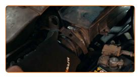
Tighten the air duct clamp.
