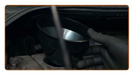
Pour new oil into the engine in the amount recommended by the car manufacturer.
