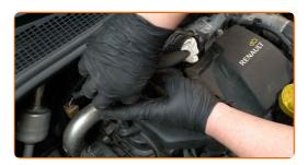
Attach the engine wiring harness. Use a flat screwdriver.
