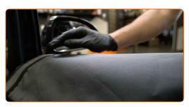
Use the masking tape to prevent plastic and painted parts of the car from being damaged.
