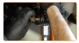
Screw in the lower fastener of the shock absorber. Use a drive socket #E18. Use a ratchet wrench.
