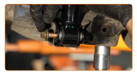
Screw in the lower fastener of the shock absorber. Use a drive socket #E18. Use a ratchet wrench.
