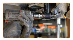
Remove the fastening bolt.
