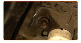
Screw the upper fastener of the shock absorber. Use a drive socket #E16. Use a ratchet wrench.
