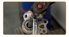
Remove the shock absorber mount, boot and bump stop.
