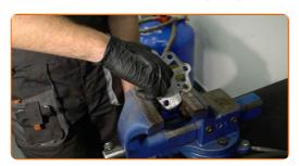
Tighten the shock absorber rod nut. Use a drive socket #18. Use a shock absorber socket DDNº6 Use a torque wrench. Tighten it to 25 nm torque.
