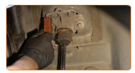
Unscrew the lower fastener of the shock absorber. Use a drive socket #E18. Use a tap wrench.
