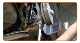
Tighten the lower fastener of the shock absorber. Use a drive socket #E18. Use a torque wrench. Tighten it to 90 Nm torque.
