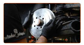
Tigten the brake drum fasteners. Use Torx T30. Use a torque wrench. Tighten it to 4 Nm torque.
