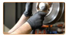
Remove the brake drum.
