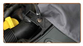
Remove the air intake pipe.
