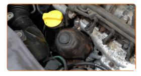
Screw in the fasteners of the protective case of the oil filter housing. Use Torx T25. Use a drive socket #10. Use a ratchet wrench.
