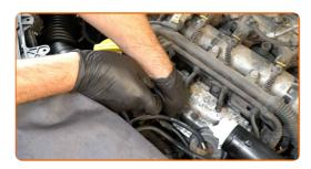
Remove the protective case of the oil filter housing.
