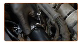
Screw in the fastener of the air intake pipe. Use Torx T25.
