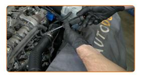
Disconnect the air intake pipe fastening. Use Torx T25. Use a ratchet wrench.
