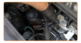
Replacement: engine oil and filter – Opel Corsa D. Tip from AUTODOC experts:
