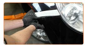
Carefully release the bumper from the fasteners.
