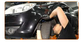
Unscrew the lower fasteners of the bumper. Use Torx T25. Use a ratchet wrench.
