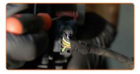
Detach the retainers and remove the bulbs from the headlight.
