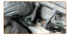
Unscrew the glow plugs. Use the spark plug socket #8. Use a ratchet wrench.
