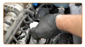
8 Detach the glow plug wiring connectors.
