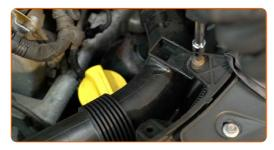
19 Install the engine cover and secure it.
