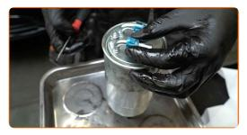
10 Remove the fuel pressure sensor.
