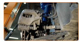
Tighten the fastener connecting the stabilizer link to the stabilizer bar. Use a combination spanner #17. Use a drive socket #17. Use a torque wrench. Tighten it to 40 Nm torque.
