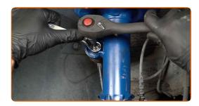
Unscrew the fastener connecting the stabilizer link to the stabilizer bar. Use a combination spanner #15. Use Torx T30. Use a ratchet wrench.
