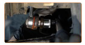
Tighten the fastener connecting the stabilizer link to the shock strut. Use a combination spanner #17. Use a drive socket #17. Use a torque wrench. Tighten it to 40 Nm torque.
