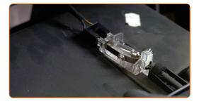
20 Screw the glove box fastening screws. Use Torx T20.
