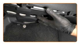
Screw in the fasteners of the bottom trim panel. Use Torx T20.
