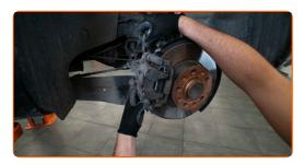
Tighten the brake caliper bracket. Use XZN #14. Use a torque wrench. Tighten it to 90 Nm torque.
