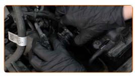
Disconnect the vacuum hose from the air filter housing.
